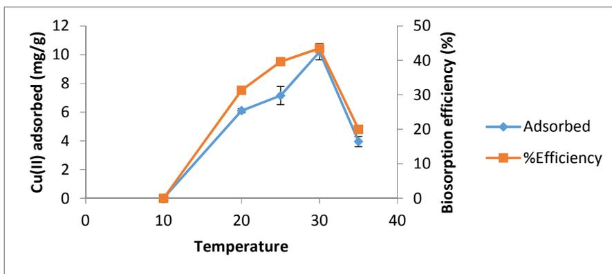
**Figure 4:** Copper (II) biosorption ( $\text{mg g}^{-1}$  d.wt) and biosorption efficiency by *Fusarium equiseti* KR706303 at different temperatures. Amount of dried biomass: 0.04 g; initial metal concentration ( $C_i$ ):  $50 \text{ mg L}^{-1}$ ; suspension volume: 20 mL; pH: 9; agitation speed: 150 rpm. The data are the mean values of 3 replicates, and the bars indicate the standard deviation of the mean.
