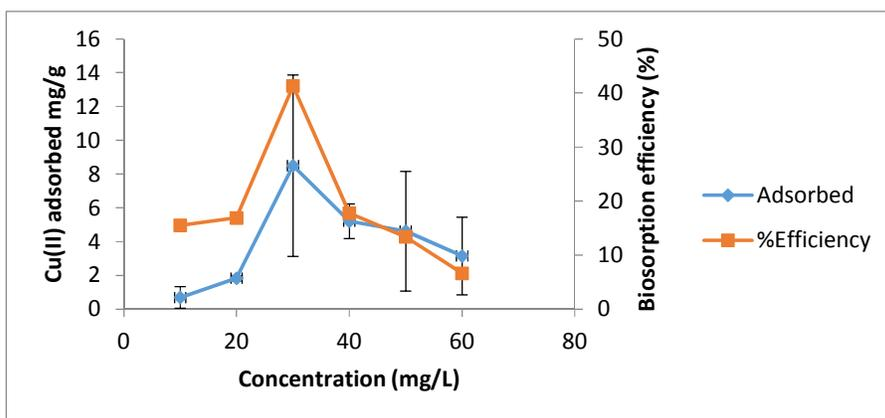
**Figure 5:** Copper (II) biosorption ( $\text{mg g}^{-1}$  d.wt) and biosorption efficiency by *Fusarium equiseti* at different concentrations. Amount of dried biomass: 0.04 g; suspension volume: 20 mL; temperature: 30°C; pH: 9; agitation speed: 150 rpm. The data are the mean values of 3 replicates, and the bars indicate the standard deviation of the mean.
