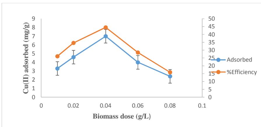
**Figure 6:** Copper (II) biosorption ( $\text{mg g}^{-1}$  d.wt) and biosorption efficiency by *Fusarium equiseti* KR706303 at different biomass dose. Initial metal concentration ( $C_i$ ):  $50 \text{ mg L}^{-1}$ ; suspension volume: 20 mL; temperature:
