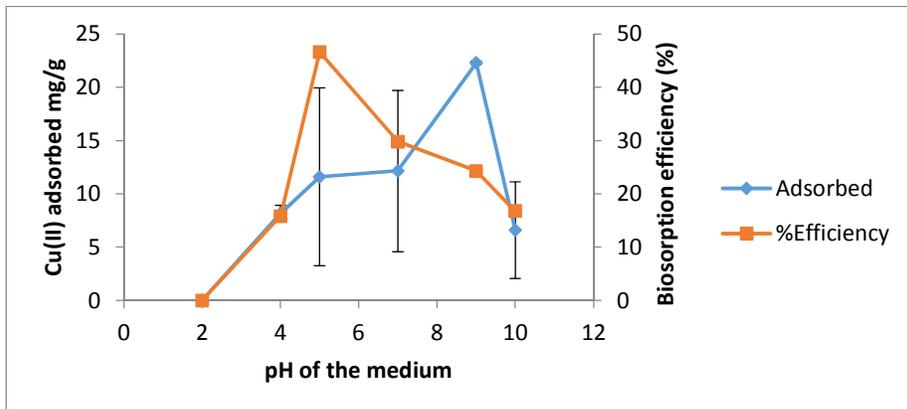
**Figure 3:** Copper (II) biosorption ( $\text{mg g}^{-1}$  d.wt) and biosorption efficiency by *Fusarium equiseti* KR706303 at different pH values. Amount of dried biomass: 0.04g; initial metal concentration ( $C_i$ ):  $50 \text{ mg L}^{-1}$ ; suspension
