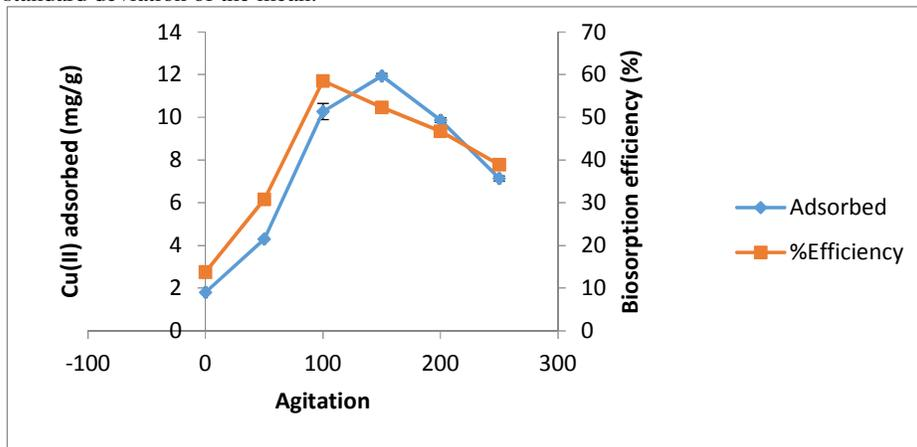
**Figure 7:** Copper (II) biosorption ( $\text{mg g}^{-1}$  d.wt) and biosorption efficiency by *Fusarium equiseti* KR706303 at different agitation speed. Amount of dried biomass: 0.04 g; initial metal concentration ( $C_i$ ):  $50 \text{ mg L}^{-1}$ ; suspension volume: 20 ml; temperature: 30°C; pH: 9. The data are the mean values of 3 replicates, and the bars indicate the standard deviation of the mean
