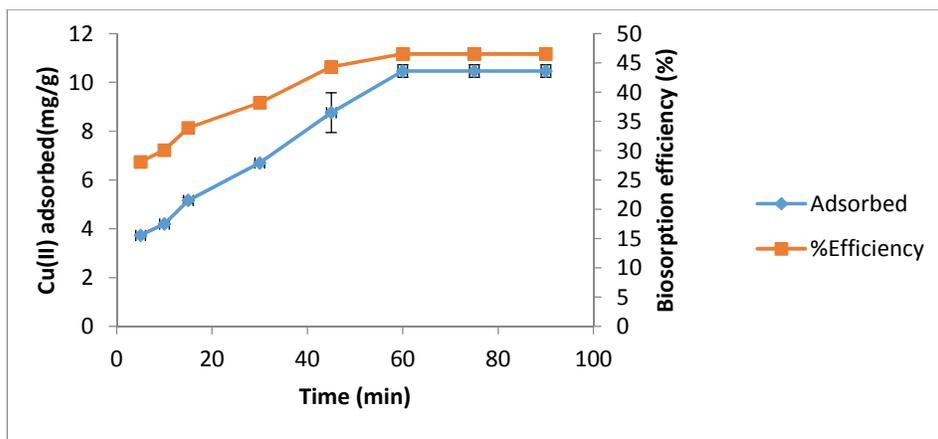
**Figure 8:** Copper (II) biosorption ( $\text{mg g}^{-1}$  d.wt) and biosorption efficiency by *Fusarium equiseti* KR706303 at different time intervals. Amount of dried biomass: 0.04 g; initial metal concentration ( $C_i$ ):  $50 \text{ mg L}^{-1}$ ; suspension volume: 20 mL; temperature: 30°C; pH: 9; agitation speed: 150 rpm. The data are the mean values of 3 replicates, and the bars indicate the standard deviation of the mean.
