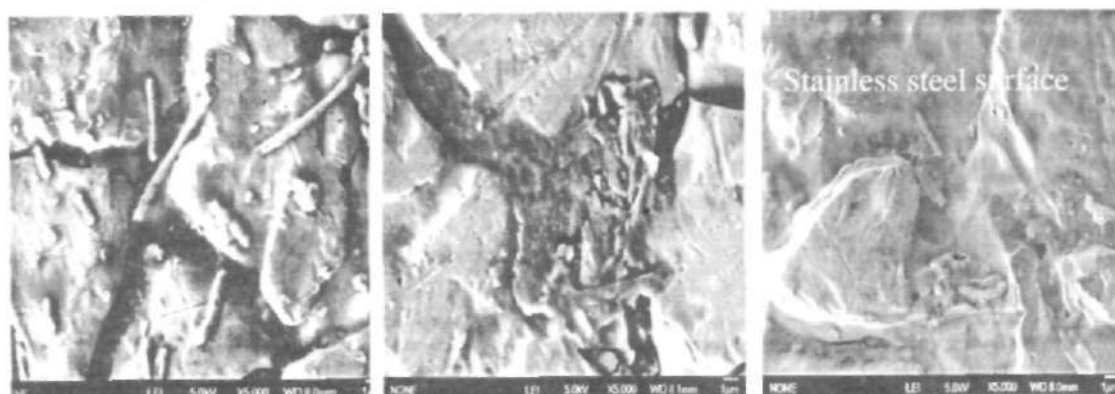
Figure 5: SEM micrographs of stainless steel coupons covered with E. coli DH5α biofilm. The images are in increasing order of magnification.
